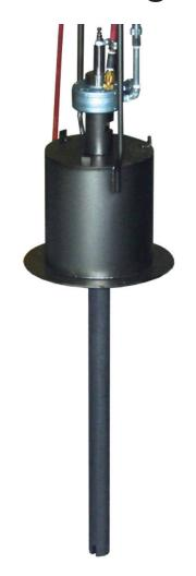
Palmer's portable rotary degasser works on the principle of increasing the surface area of an inert gas exposed to the metal: The greater the surface area, the faster the degassing will be.
